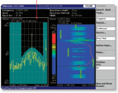
Using the Frequency Mask Trigger and Spectrogram to determine if interference with
